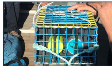
SMELTS gear also uses “on-demand release,” but with an inflatable bag instead of a line.
