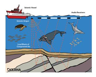
Seismic airgun blasting is a dangerous and extremely loud process used to search for potential oil and gas deep below the seafloor.
