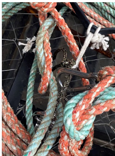
Figure 6: Rotten cotton connecting the release line to the bungee allows provides a backup release mechanism for the fishing line and floats if the primary release mechanism fails.
