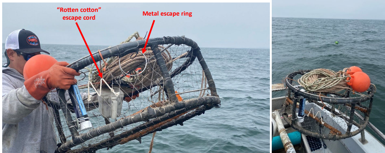
Figure 5: Configuration including degradable “rotten cotton” and steel escape ring installed on the side of the trap.
