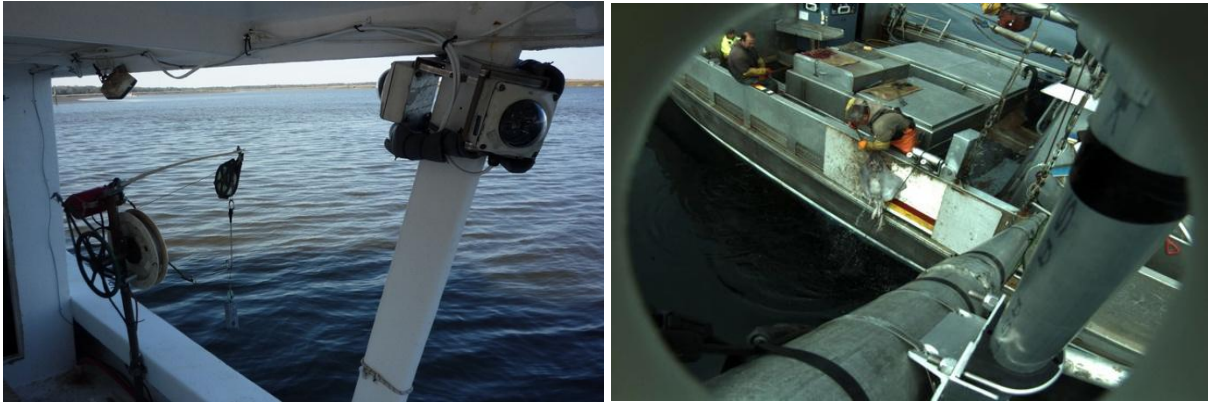
Images courtesy of NOAA Fisheries. Electronic monitoring systems installed on fishing vessels.
