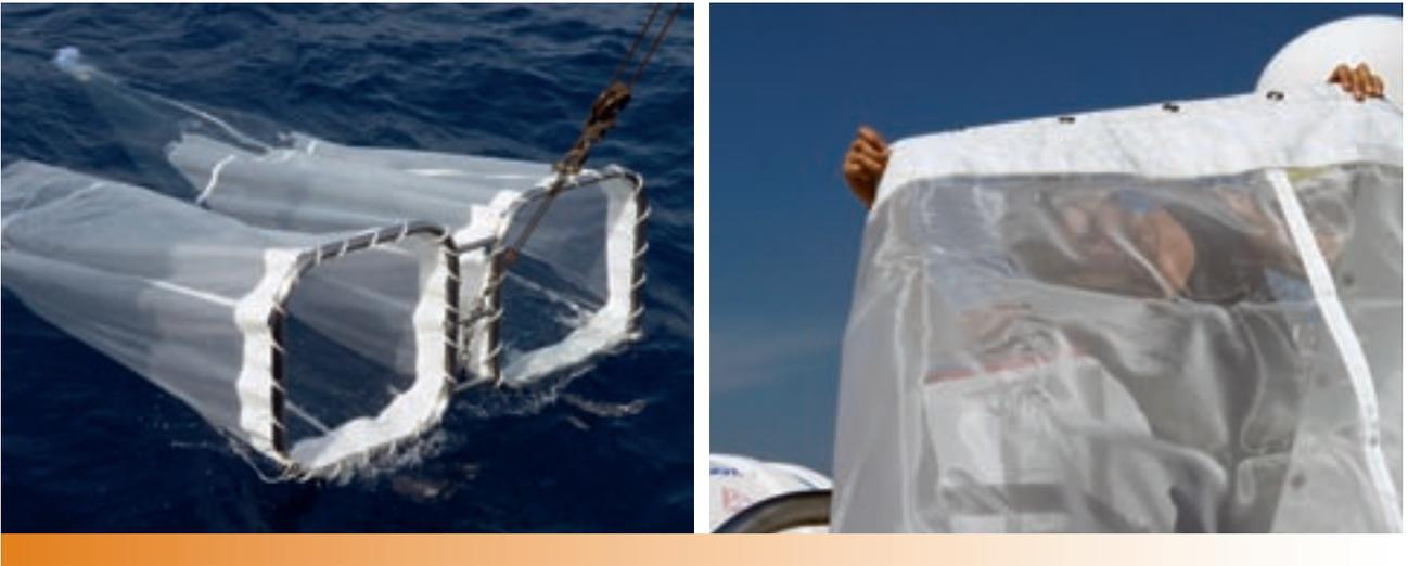
Figure 2, 3: On the left, the bongo 90 net used for sampling; on the right, the 500  $\mu\text{m}$  mesh-size net. © OCEANA/ Keith Ellenbogen
