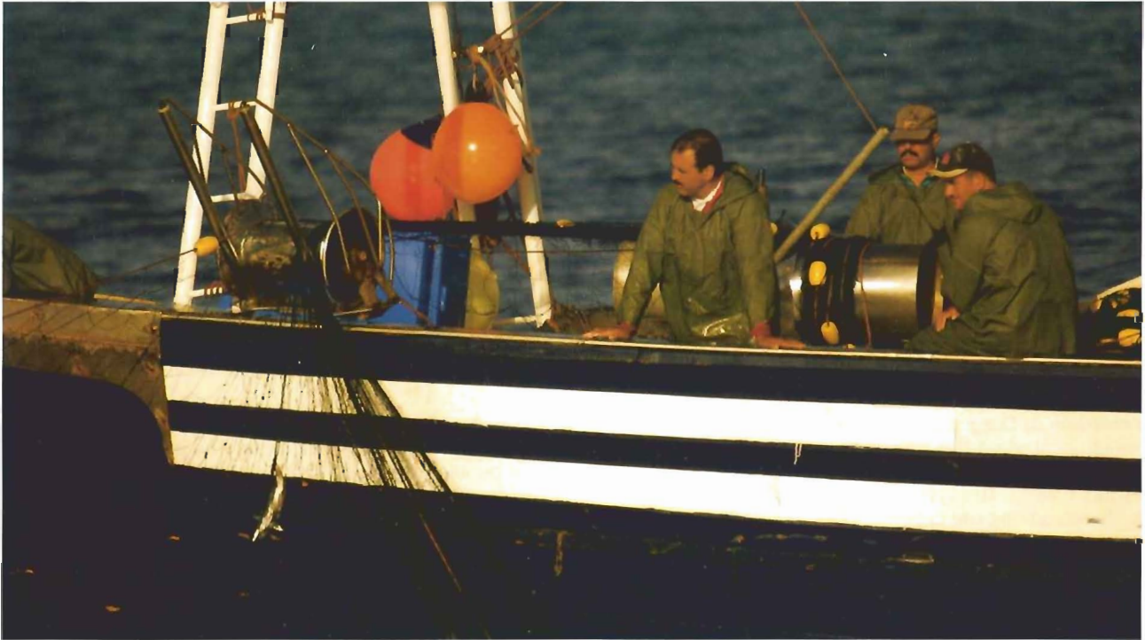
© OCEANA/Juan Cuctos. Net hauler and winch mounted on a Moroccan driftnetter. Alboran Sea, August 2006.
