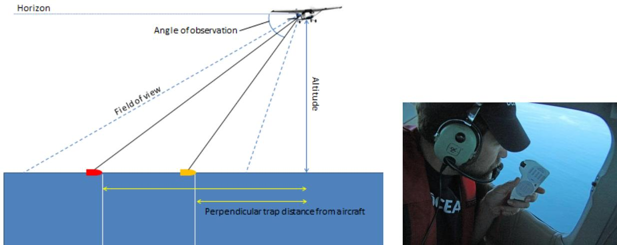
**Figure 3.** Left: Diagram showing how angle of observation can be used to calculate perpendicular distance of buoys from the aircraft transect track line. Right: Observer Dr. Geoff Shester views traps from the window of the aircraft using a clinometer to determine the angle of each observed trap relative to the aircraft.
